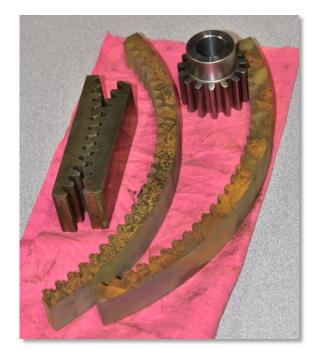
Charlie Reiter had a brass heat pump. He also showed internal gear segments for tractor wheels that were cut from flat stock using a water jet.
