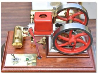
John Gilmore's GEM1 engine was started after some years of non-use. The gas tank was filled with a gelatinous green "gunk" that required meticulous cleaning.
