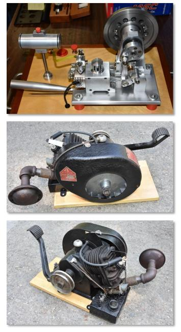
He then showed us a second "First Pops", at least after a major repair. It was the "Johnson 4-Cycle Iron Horse" discussed at our last meeting . Paul Denham machined a very complex helical gear using a four axis CNC mill. This was to replace a badly damaged and stripped out gear. The ignition points were badly pitted and required a polishing on Dwight's diamond wheel. Following the meeting it fired up nicely after a few kicks.
