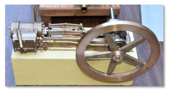
Jim Piazza has finished a PM Research #1 Drill steam engine. The kit is of bronze and finished nicely by Jim. He reports that it runs beautifully and is now waiting for a "brick sheet" (also from PM research) for the base. He will also fit studs with hex nuts for the head as well as brass oil cups. He modified the eccentric, and changed to a built-up crankshaft after discarding the cast shaft blank provided in the kit.
