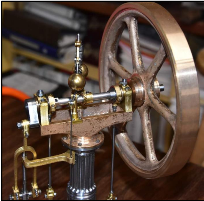
Close view of the fly-ball mechanism.
