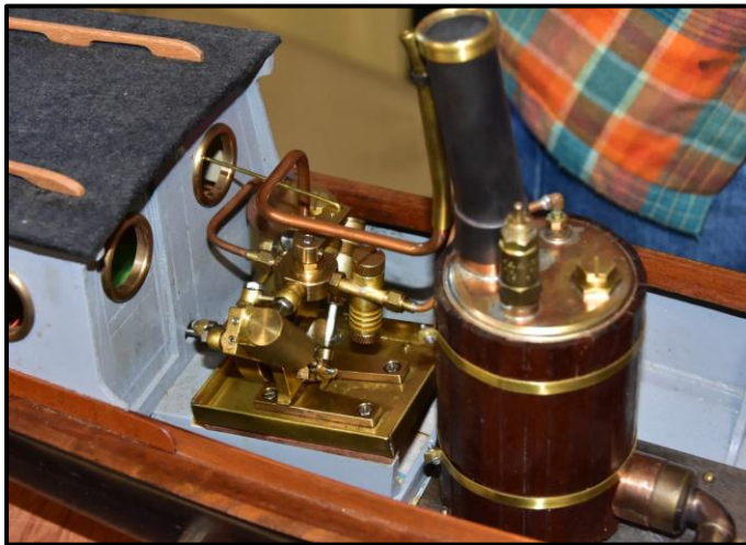
Closer view of steam engine and boiler.
