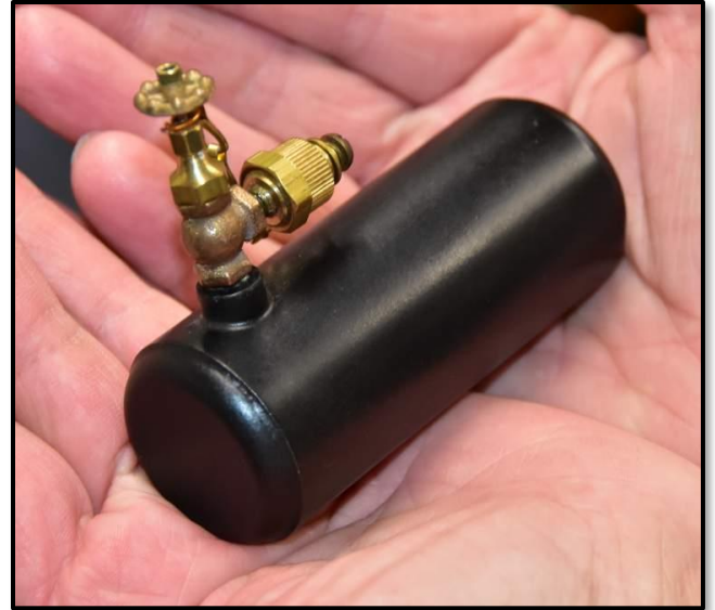
Charlie fabricated the fuel tank to be easily removable, for ease in filling it with propane.
