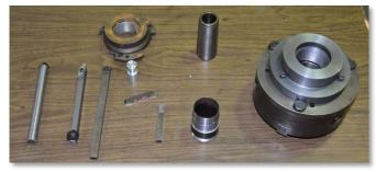
Jerry Franklin has a 1919 14-inch lathe and managed to break the cast iron back plate adapter plate for his 3-jaw chuck. Since his 2 1/8 – 8 spindle is not common, he undertook a shop made replacement. This was his first adventure in single point internal threading. He had the new adapter mounted on the chuck and it looked very nice. Not clear how he was able to turn the new adapter in his chuck still using the broken adapter.
