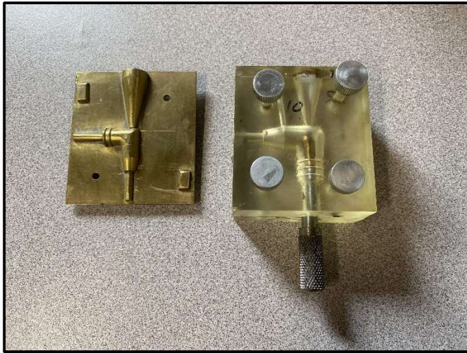
Left: pattern used to create molding fixture. Right: two-part molding fixture cast with resin, including stainless jig used to hold wire in correct orientation for molding. Wire/clip/jig assembly is placed in mold, liquid urethane is poured into conical hole in top of mold. Multiple molding fixtures can be cast from the pattern, permitting production of multiple rubber spark plug boots at the same time.
