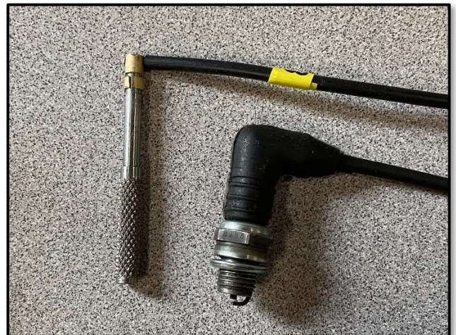
Right: finished molded spark plug boot. Left: 10000 volt insulated wire soldered to spark plug clip, with stainless jig. The jig holds it in the molding fixture, as well as serving as a space-filling core that creates the inner hole which fits over the spark plug.
