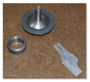
Dwight furnished a device for compressing the rings and reinserting the pistons. He also had a fixture using wet and dry sandpaper for ring gapping.
