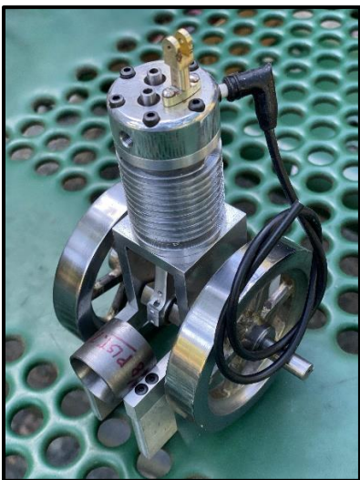
Dwight latest model engine, the GEM2. Note the molded rubber spark plug cap.
