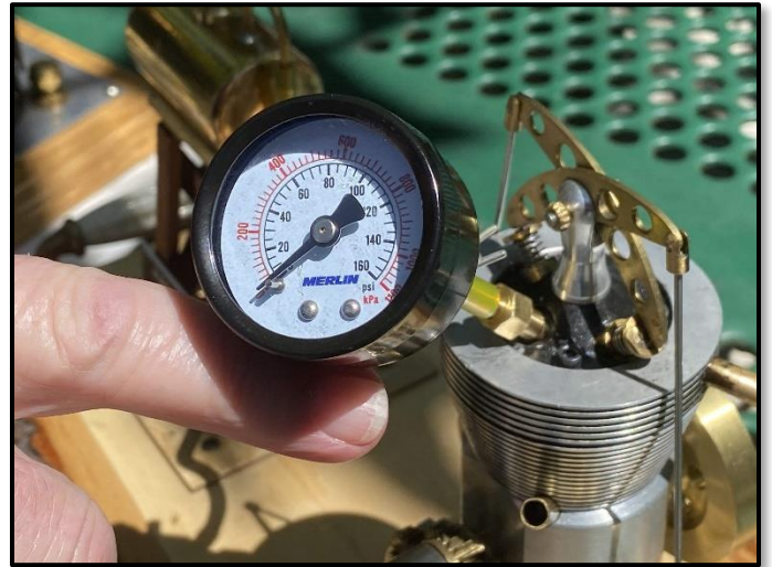
George shows cylinder pressure measurement gauge
