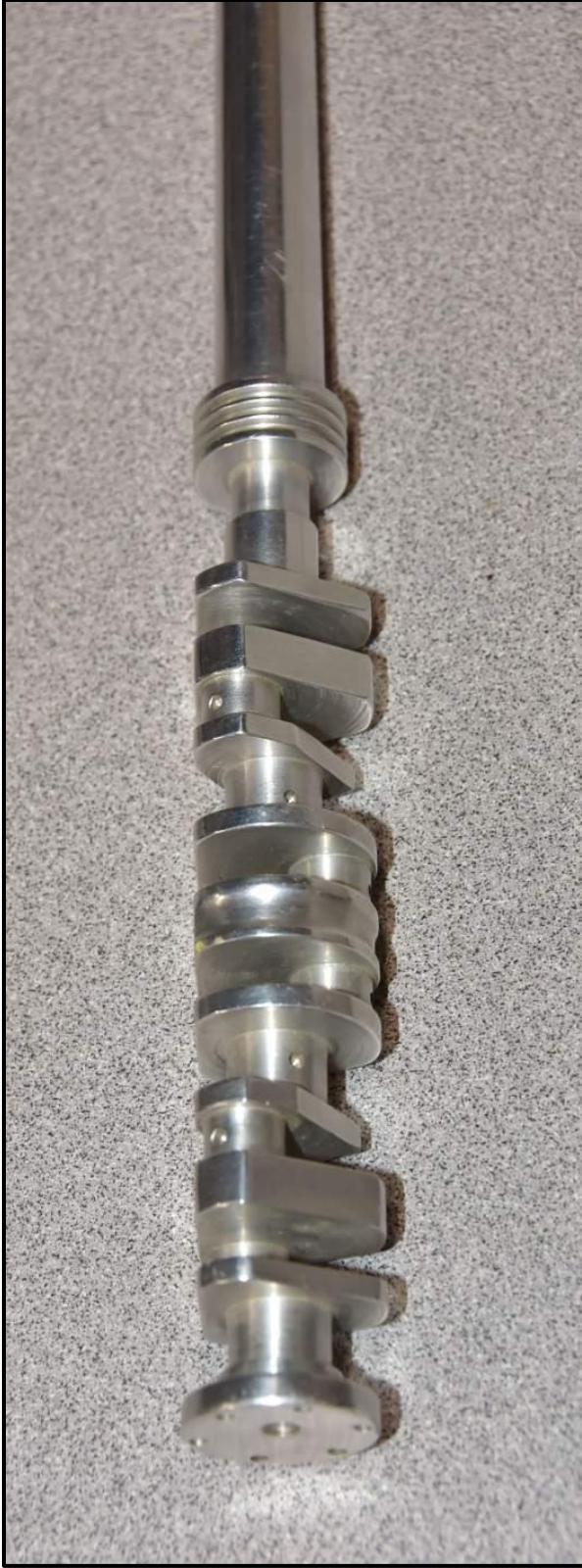
Mike Byrne's aluminum pointing rod. The handle was a four-cylinder engine crankshaft.
