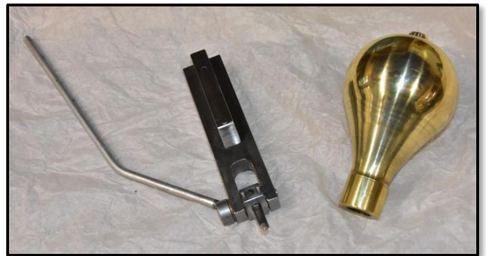
Charlie explaining how he created a hollow brass air reservoir.
