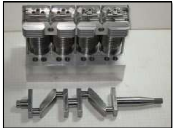
Newly finished crankshaft for Peter's De Havilland Cirrus aero engine along with pistons and block.
