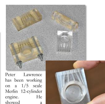
distributor parts machined in two parts in order to accommodate wiring geometries.
