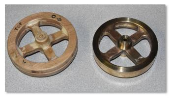
Wes Wagon brought a bronze fly wheel with casting patterns he made in a recent foundry class at the Crucible in Oakland. His next step is to build an engine to go with it.
