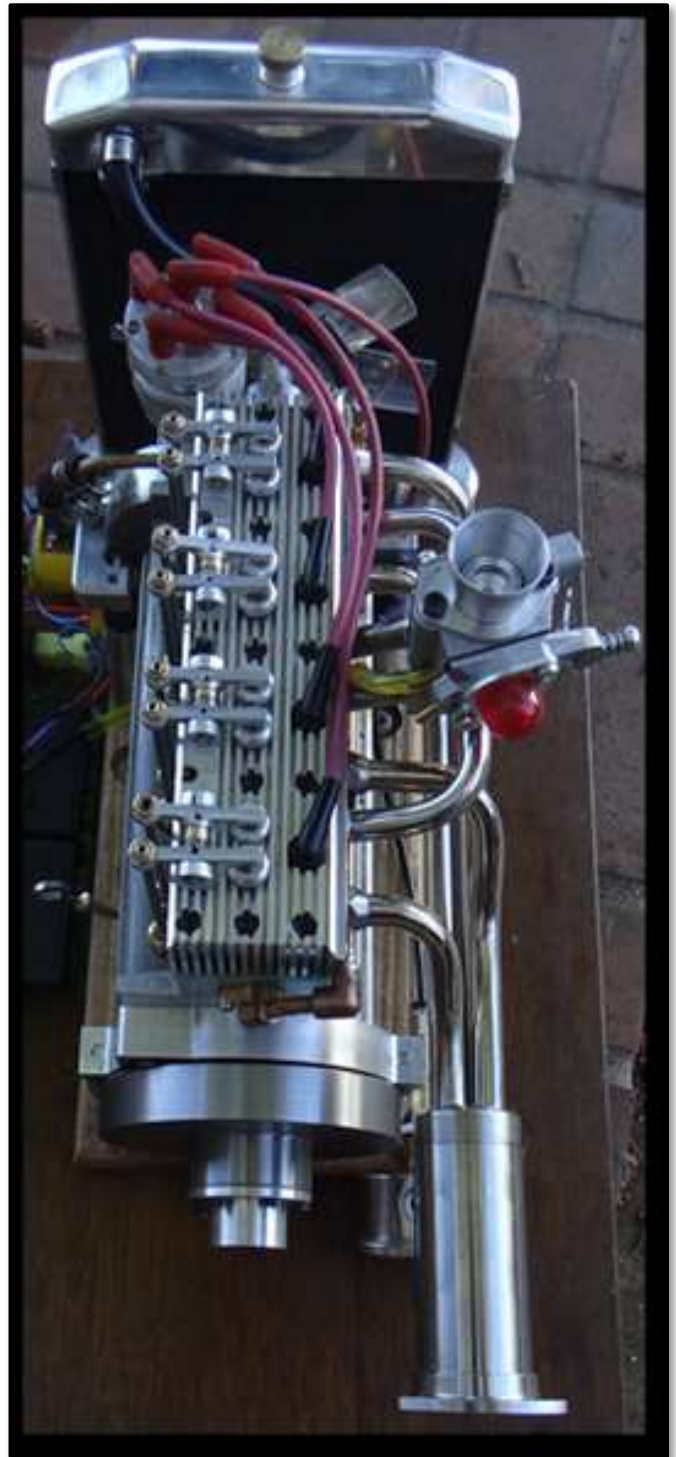
The intake/exhaust tubing is made from thin-wall stainless steel, carefully bent and polished.
