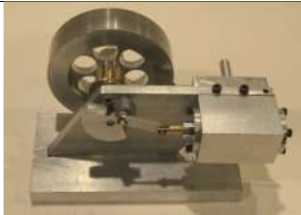
Mike's reverse engineered horizontal (for bar stock) double acting spool valve
