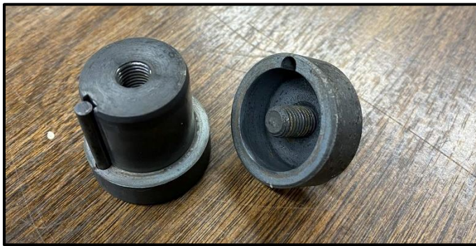
This fixture holds multiple rings during the annealing process. The rod embedded in the side of the inner cylinder spreads the ring gap a precise amount, holding it there during the heat treatment process. The notch in the inside of the cap permits the cap to fit snugly, holding the rings in an orderly stack.
