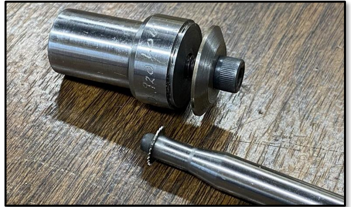
Fixture for slotting oil control rings
