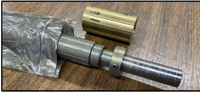
Dwight's lapping device, with diamond paste saved for next time
