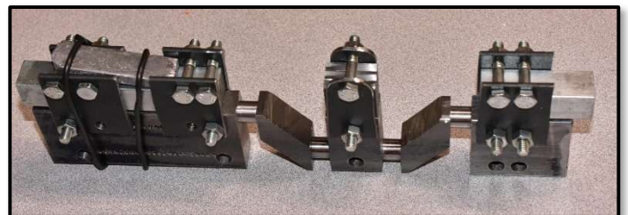
Peter Lawrence's crankshaft lathe turning fixture.
