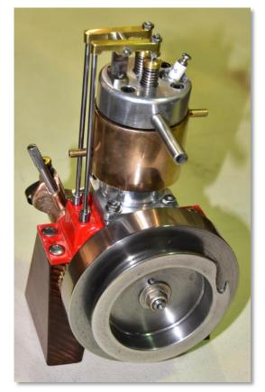
Dwight has be reworking a single cylinder throttle governed vertical boat engine of uncertain origin. Dwight shared hints on machining a tapered collet for the flywheel and suggestions for machining and lapping valve guides. Dwight also offered club members spare rings in a variety of sizes. Dwight believes it is prudent to always make some "extras".
