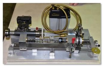
Peter Lawrence has been assembling a cam grinder and brought it in to show progress including a new master with 120 degree lobe seperation. His primary motivation is his Merlin V12 project. With 4 valves for each of twelve cylinders, that is a lot of cam lobes to grind (two cams of 24 lobes each). Peter recommends use of a mister to reduce dust.
