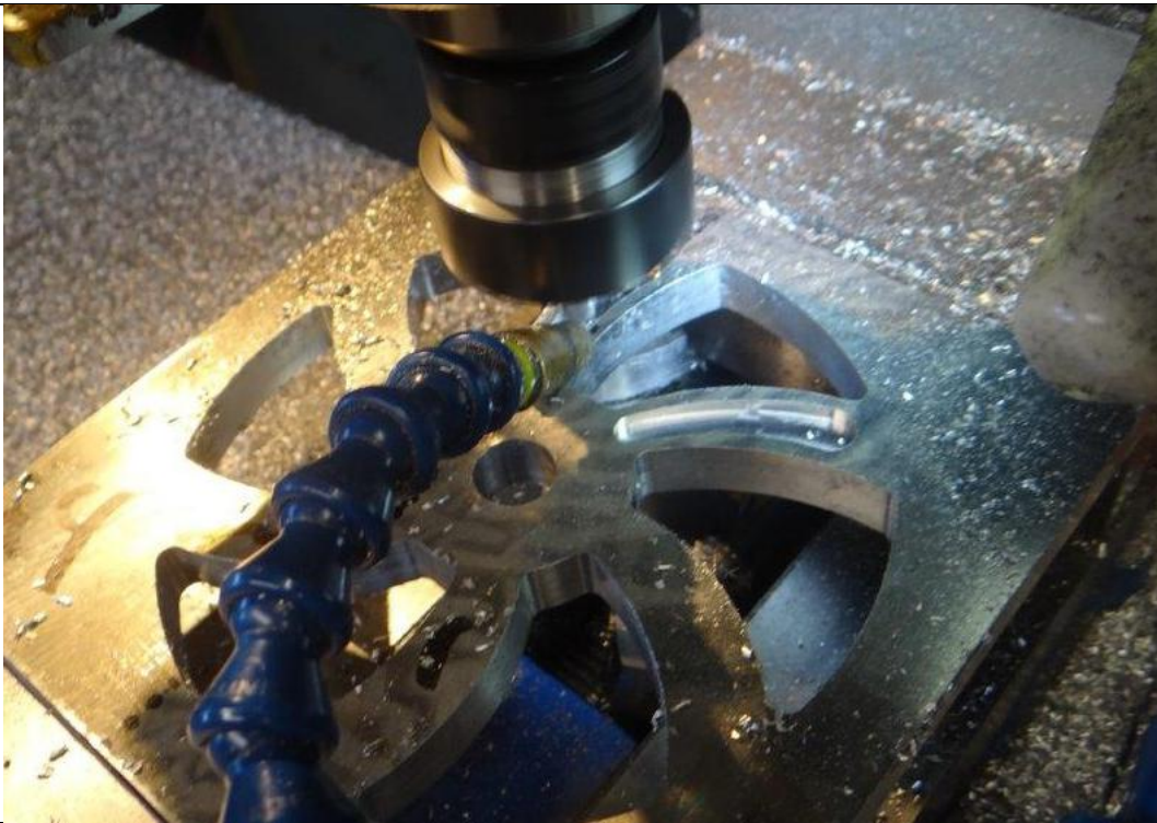
Flywheel spoke and hub machining underway after new X-controller installed
