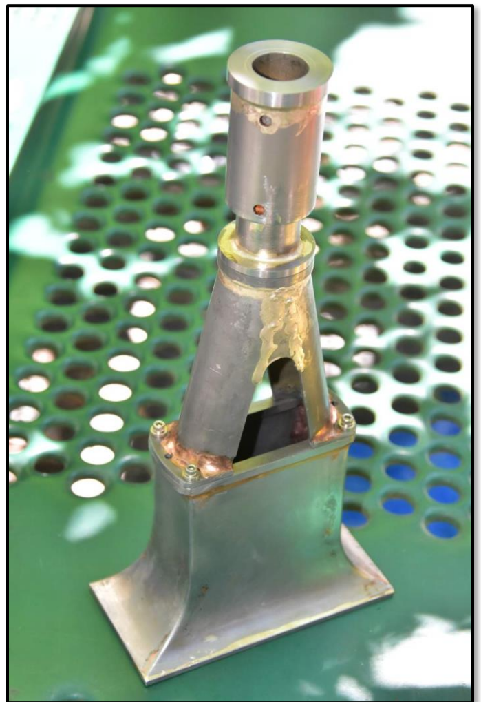
Brazing, an efficient way to join thin metal pieces
