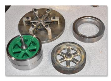
Dwight Giles brought his fixtures for silver soldering flywheel spokes and showed examples of post silver soldered and finished flywheels. Details were published in the Model Engine Builder volume 31.
