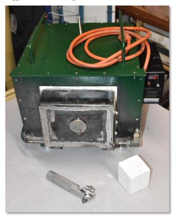
Tom Blanchard brought in a shop built an electric heat treat furnace and discussed fire brick cutting and heater coil winding.
