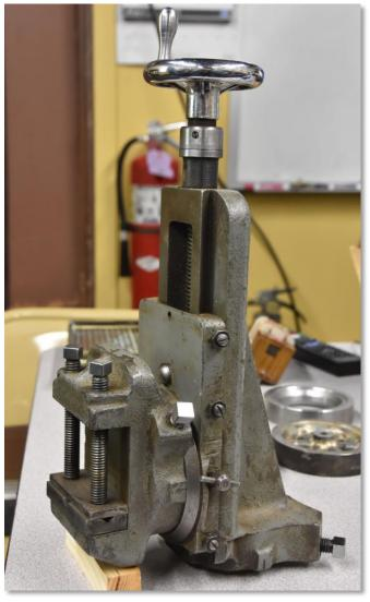
Dwight also brought in a low tension ignition coil, a radiator, and a rebuilt milling attachment for an Atlas lathe.
